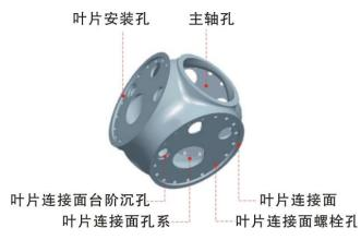
叶片安装孔: mounting hole of blade
